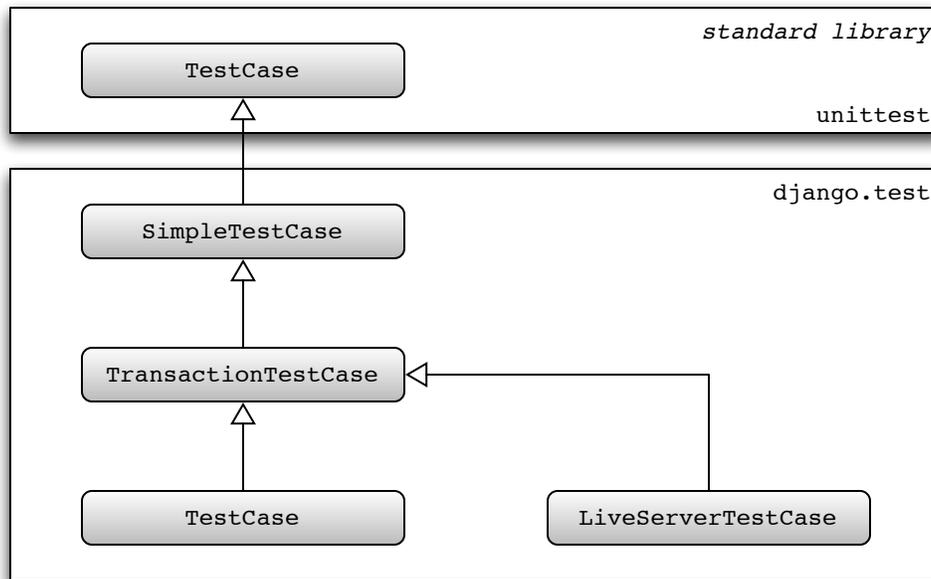
Fig. 3.1: Hierarchy of Django unit testing classes
